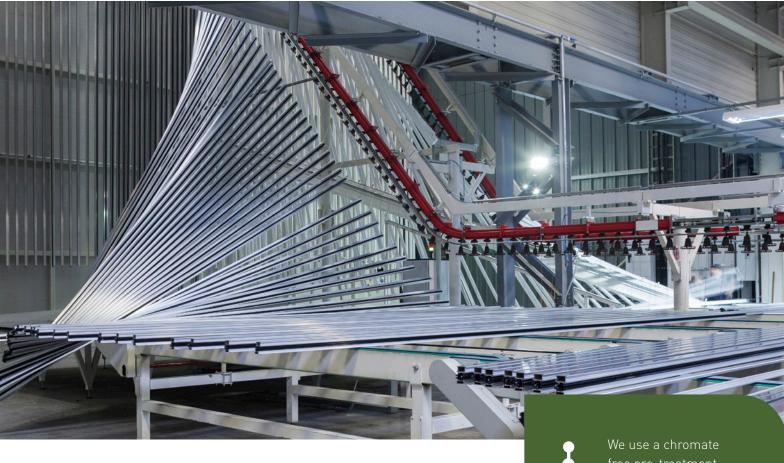
Above – The conveyor is feeding in to one of our two vertical powder coat paint lines..
